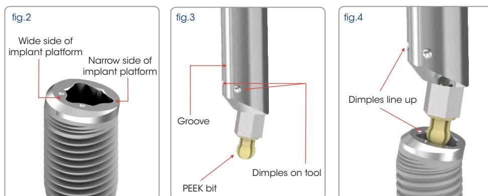
**Important:** The PEEK bits (I-PBIT-L18 / L20) should be replaced on a regular basis. General wear & tear are to be expected with regular use. (Items sold separately)
